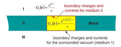
Fig. 1. Boundary element method approach to the transmission through a small hole. The problem is solved in terms of magnetic boundary charges and currents distributed around the hole boundary. See text for more details.
