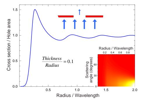
Fig. 2. Transmission cross section of a cylindrical hole in a perfect-metal slab as a function of the hole radius. The slab thickness is 0.1 times the radius. The cross section is normalized to the area of the hole, and the radius is normalized to the wavelength. The incidence of the light is perpendicular to the slab. The contour-plot inset shows the polar angle distribution of transmitted light as a function of hole radius (brighter regions stand for higher transmission intensity).
