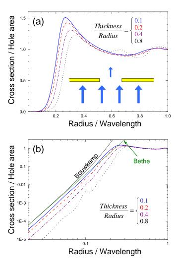
Fig. 3. (a) Transmission cross section of a cylindrical hole drilled in a perfect-metal film as a function of the hole radius for different ratios of the slab thickness to the radius (see labels). The light is coming perpendicular to the film. (b) Same as (a) in log – log scale and compared with the asymptotic formulas of Bethe (Ref. [7]) and Bouwkamp (Ref. [8]), which are valid for vanishing thickness [see Eq. (2)].
